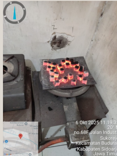
Pict 14. Check the briquette dryness with burning test
